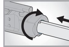
Remove carbon from 2 interior bolt carrier surfaces in one operation
