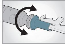
Scrape inside & outside of bolt tail and bolt tail shoulder in one operation
