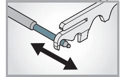
Quickly clean both diameters of firing pin
