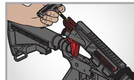
Quickly and perfectly aligns the cleaning rod with the bore without rubbing on the bore throat
