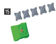
Insert desired ammount of springs to set trigger weight. Max. 5 springs possible. After adding or removing springs choose fitting buffer plate.
