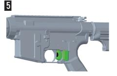
Secure trigger switch with magnetic side plate
