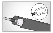
Use mop to remove loosened fouling from bore
