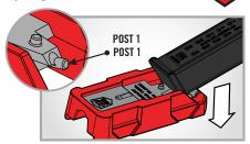
Step 1: Place rubber overmolded base on table, insert post 1 into magazine release port on bottom of base plate, then lever downward to crack loose base plate.
