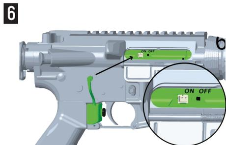
Connect cable of trigger switch with WLB15 and switch main switch to "ON".
