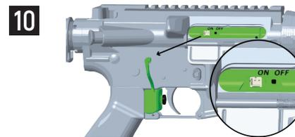
Main switch to ,OFF". Unplug cable. Remove side plate of trigger switch.
