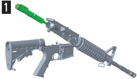
Remove original bolt carrier group. Guide WLB15 into receiver laser tip forward
